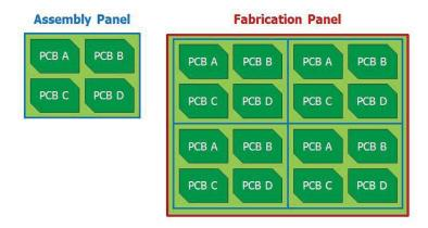
*Figure 7: In actual fabrication, the assembly panel is made four-to-a-set on the fabrication panel, which is then separated into individual boards.*
