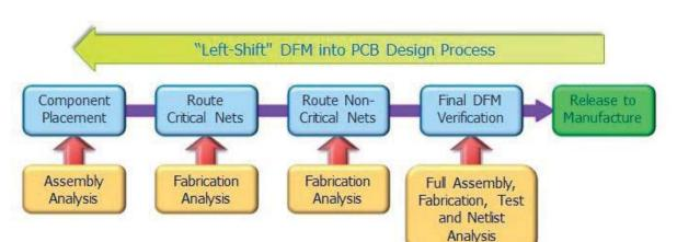
Figure 3: Concurrent engineering process, effectively "left shifting" DFM into the very beginning of the PCB design task.
