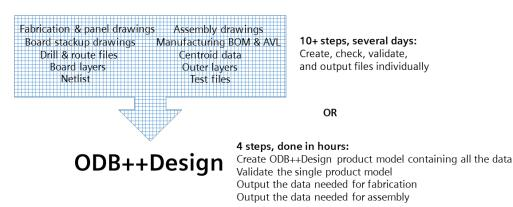
All fabrication and assembly data contained in one data model
