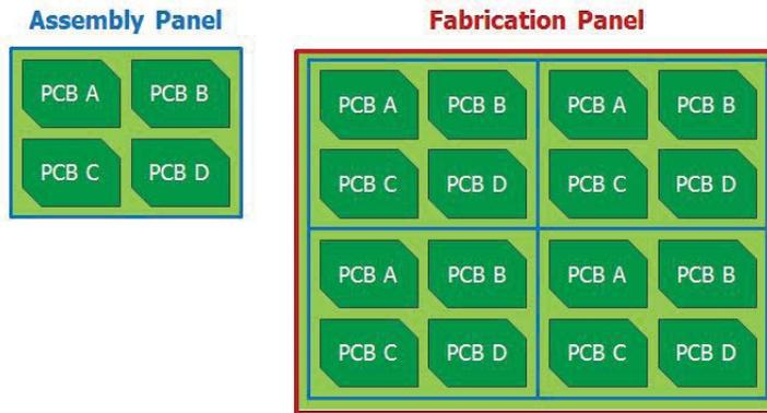
*Figure 7: In actual fabrication, the assembly panel is made four-to-a-set on the fabrication panel, which is then separated into individual boards.*
