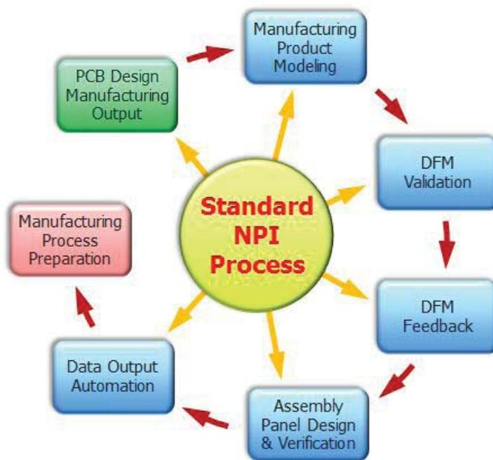
Figure 1: Standard New Product Introduction process for PCB-based products.
