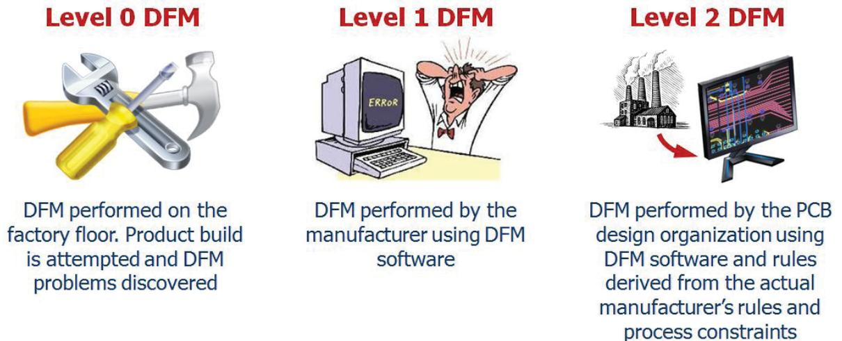
**Level 0 DFM** is performed on the factory floor where the product build is attempted and DFM problems are discovered. This method of DFM verification is very time-consuming and expensive with material wastage and production labour costs at a premium.
