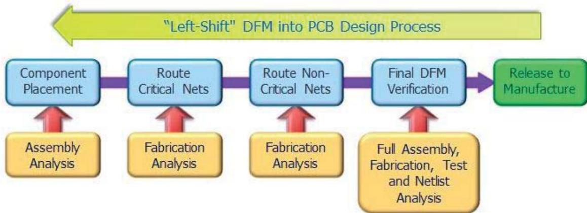
Figure 3: Concurrent engineering process, effectively "left shifting" DFM into the very beginning of the PCB design task.
