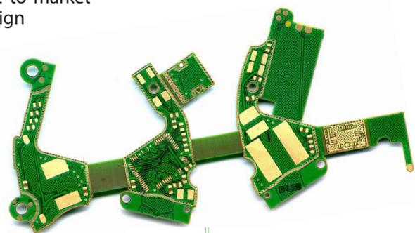
*ODB++Design now includes explicit modeling of flex and rigid-flex circuits and can convey dimensioning data.*
